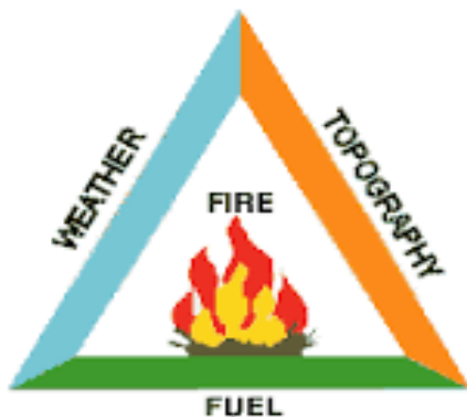
Figure VI - 9. Fire Behavior Triangle. Fire behavior characteristics are influenced by fuel, weather, and topography.
